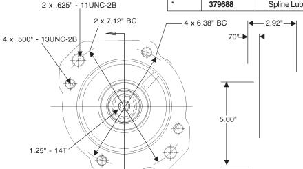
Note: \* Not required for Wet Spline \*\* Wet Spline Only
