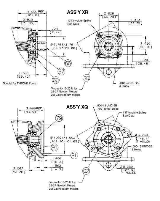
Note: "RA" and "RB" Flanges Rotate in 30º Increments
